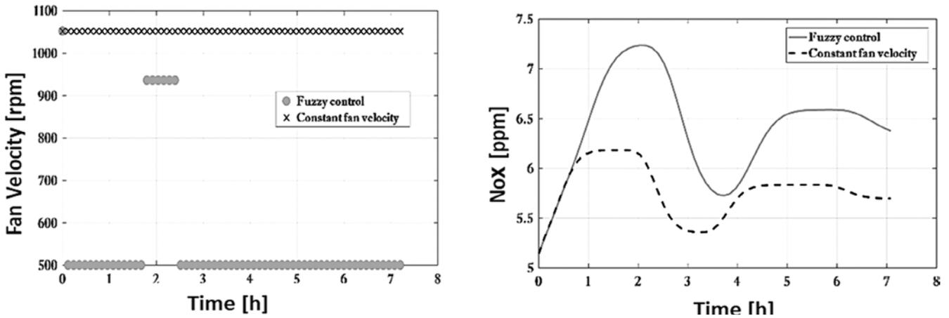
Fig. 4. Comparison between fuzzy control and constant velocity in the application to tunnel excavation.
