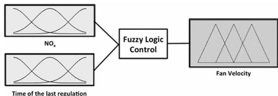
Fig. 3. Schematic of the fuzzy logic algorithm for ventilation control.
