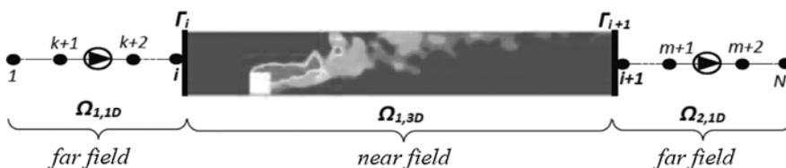
Fig. 5. Schematic representation of a multi-scale structure for tunnel ventilation analysis.
