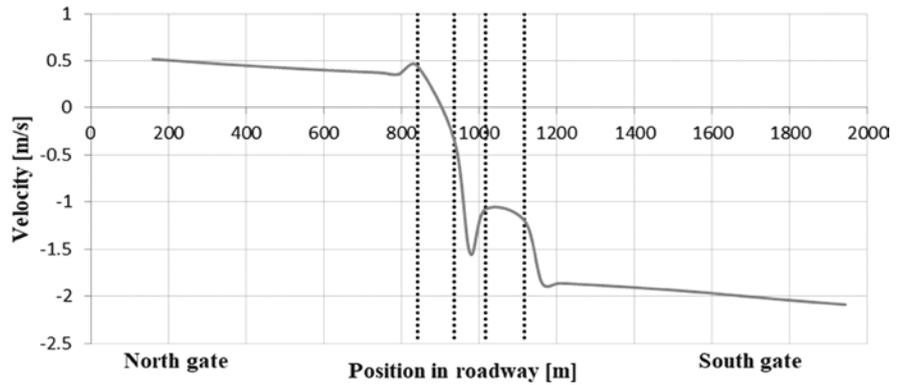
Fig. 6. Mean longitudinal velocity in the roadway in the re-design configuration.
