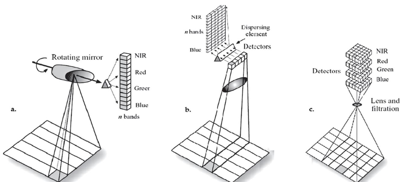
Fig. 2. Types of hyperspectral sensors: (a) whiskbroom, (b) push-broom sensors, (c) full-frame sensors (adapted from Adão *et al.*, 2017).
