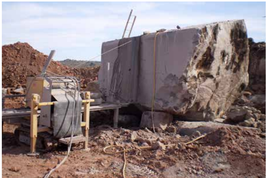
Fig. 3 – Block sawing by diamond wire in an ornamental basalt quarry.
