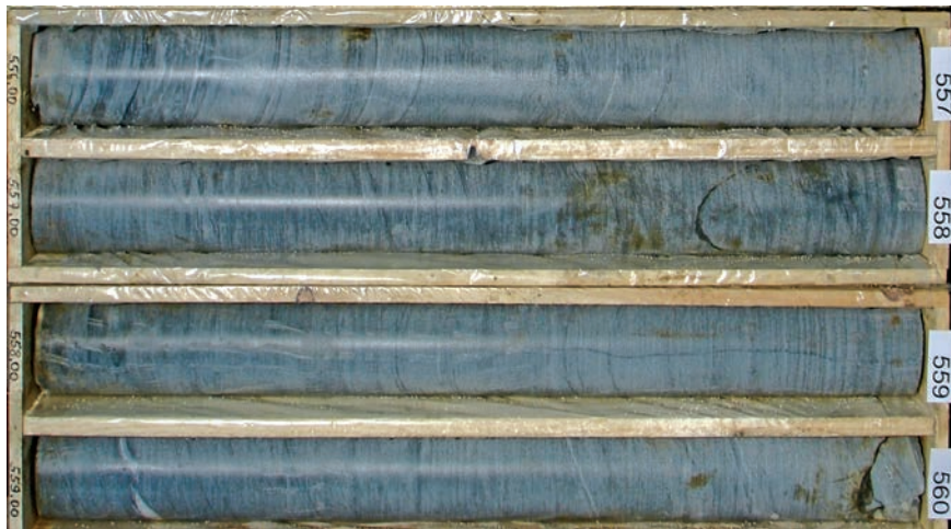
Fig. 4 – Drill core from the Hochstegen marble with RQD equal to 100%, no dissolution and discontinuities.
