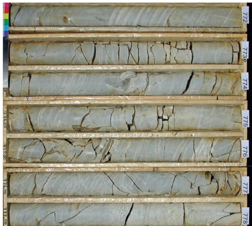
Fig. 3 – Marble with partly solution-extended fissures, e.g. 772.3 to 772.8 m.
