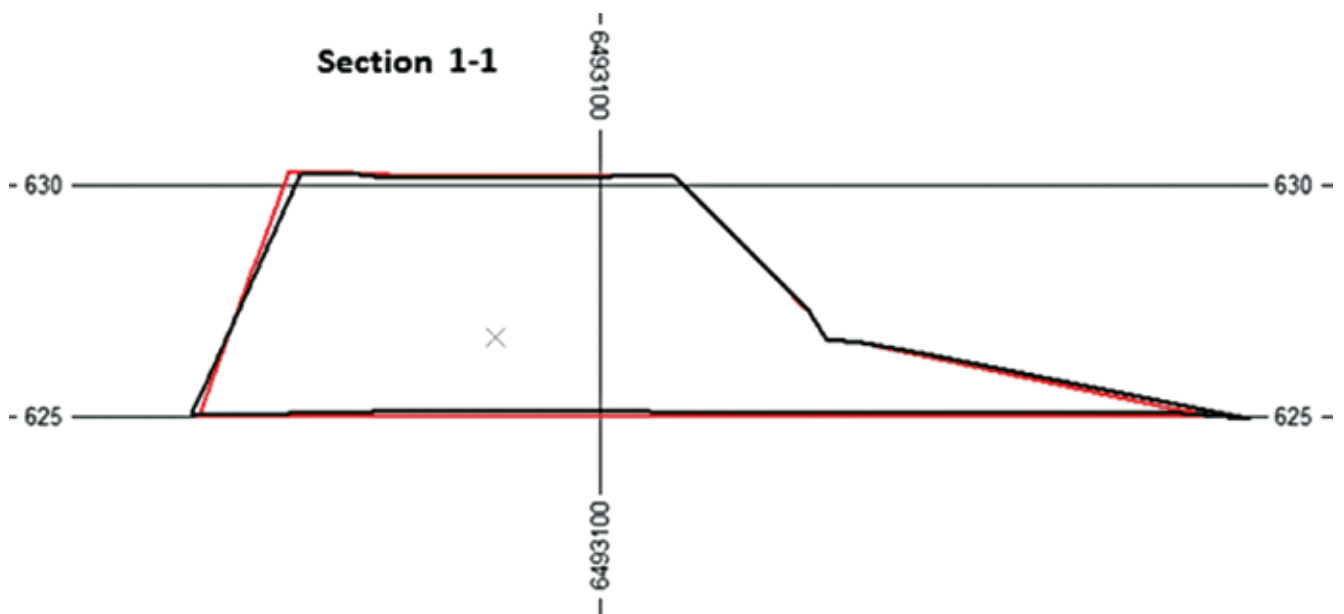
Fig. 8 – Deviations from the project during grade planning (section 1-1). Source: Compiled by the authors.
